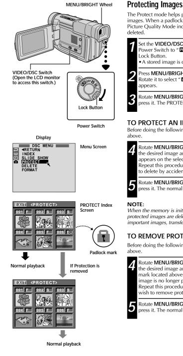
The Protect mode helps prevent the accidental erasure of images. When a padlock mark is displayed next to the Picture Quality Mode indication, that image cannot be
